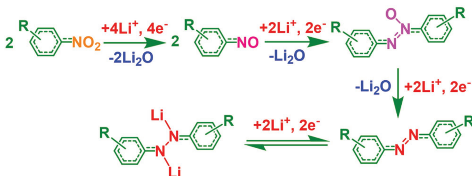
Scheme 2. Reaction mechanism for nitro-based organic materials.
