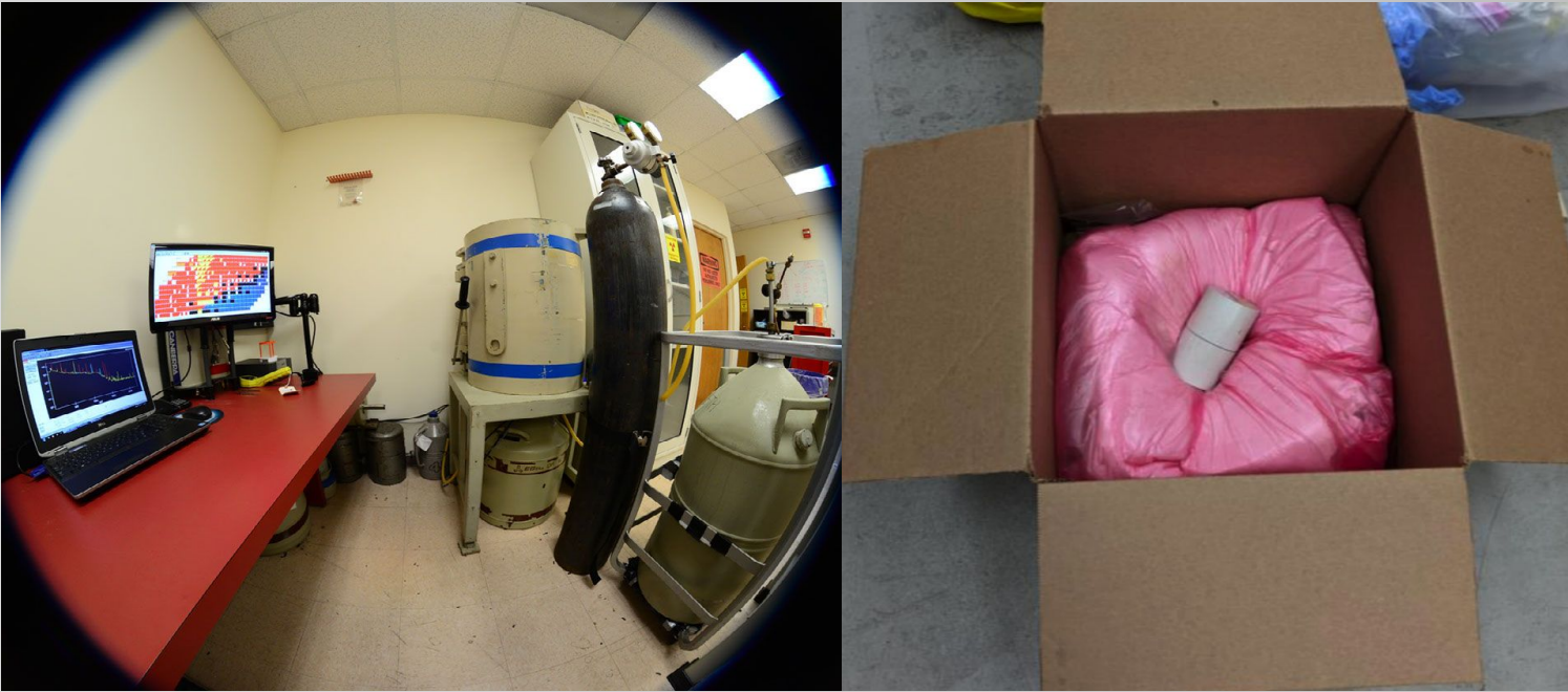
Above Left: A High Purity Germanium gamma spectrometer at the University of Maryland Radiation Facilities. Above Right: An activated Ytterbium Oxide sample packaged for shipping. Below: A graph of reactor power as the Ytterbium oxide samples were inserted into the core. The power trace clearly shows the prompt drop in reactor power that was used to calculate the reactivity worth of the samples
