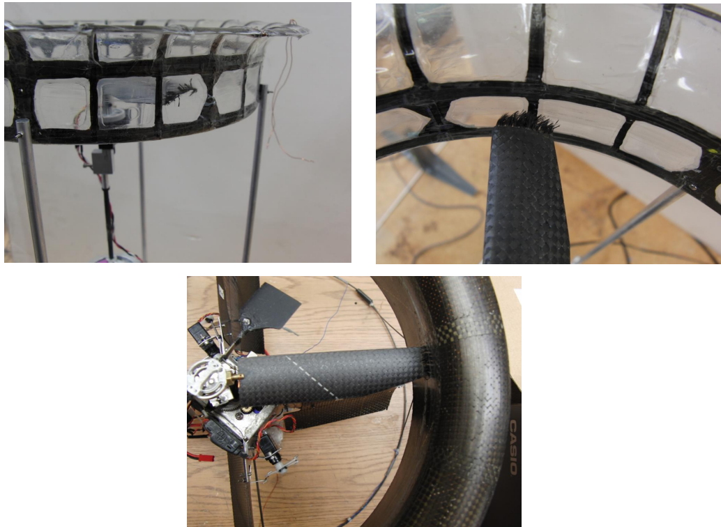
Figure 2.63: Brushes incorporated in blade tips to improve performance
