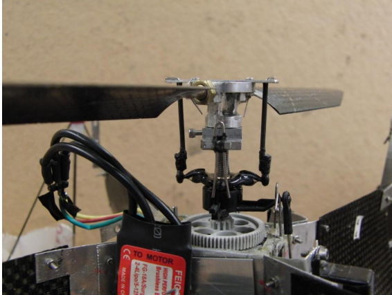
Figure 5.49: Swashplate with cyclic travel of \pm 10^\circ
