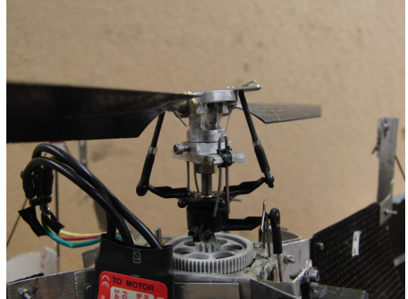
Figure 5.50: Swashplate with cyclic travel of \pm 15^\circ
