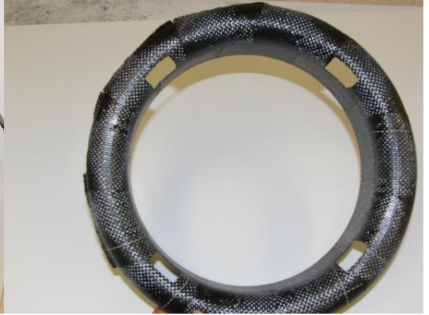
Figure 5.33: Shroud vent design
