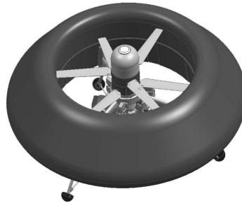
Figure 1.26: Shrouded rotor UAV prototype by Avanzini et. al. [144]
