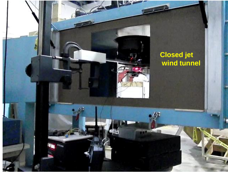
Figure 6.12: Closed jet wind tunnel set-up
