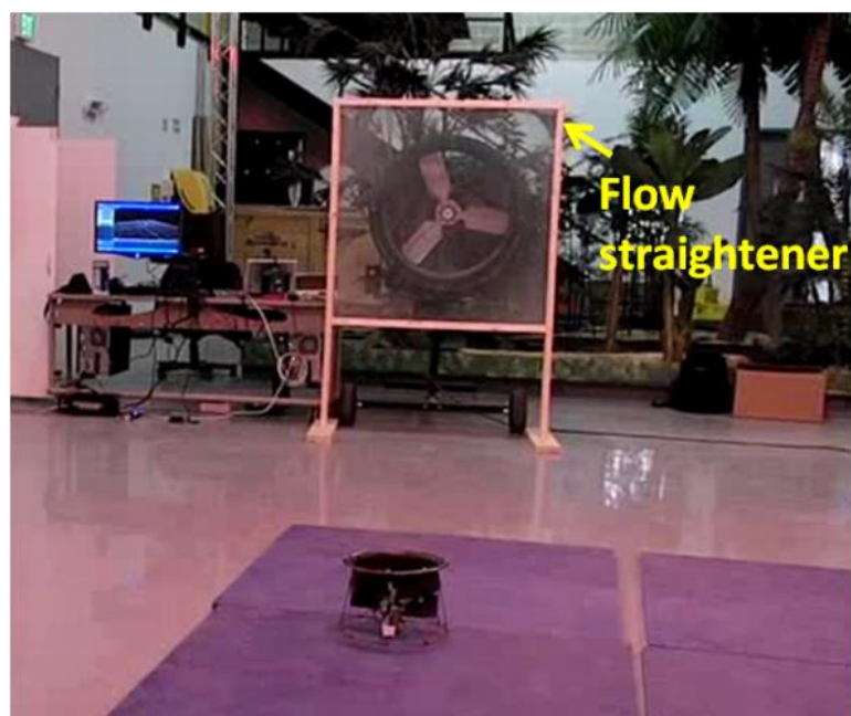
Figure 6.29: 0.75 m diameter fan gust setup
