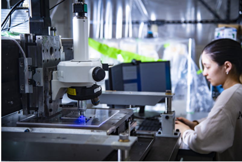
Figure 47: High resolution automatic optical microscope scanning system (PTS) for the nano-tracking with the nuclear emulsion.
