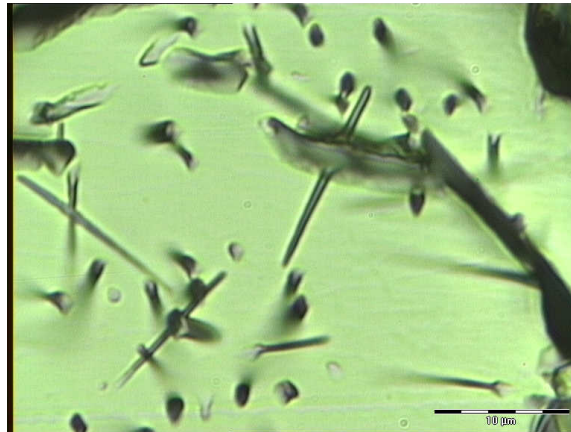
Figure 3: Etched spontaneous fission tracks in apatite visualized by optical microscopy. Apatite samples obtained from southern Uralides, Russia [93].
