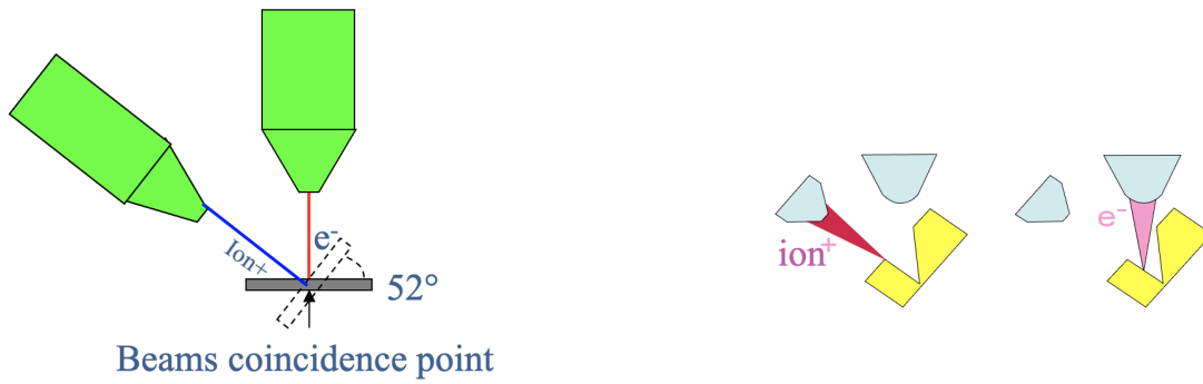
Figure 25: Schematical drawing showing the geometrical setting of a dual-beam FIB.
