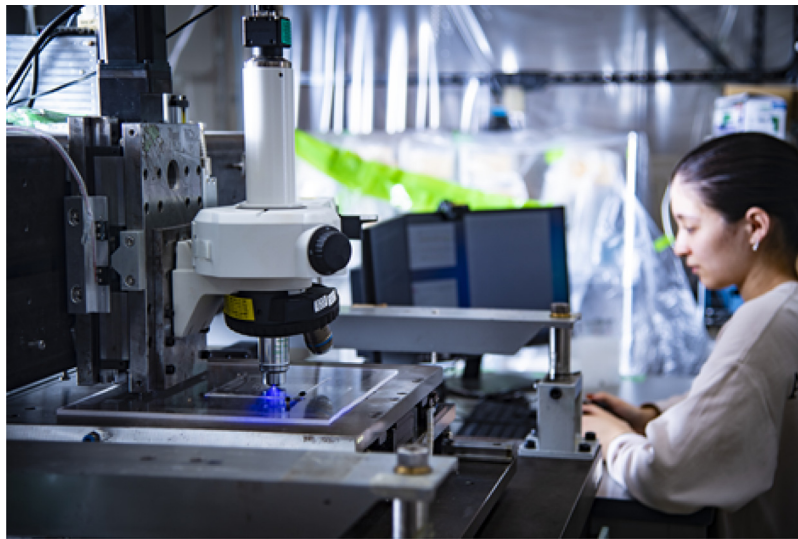
Fig. 48. High resolution automatic optical microscope scanning system (PTS) for the nano-tracking with the nuclear emulsion.
