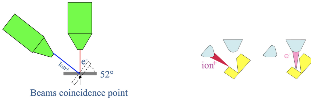
Fig. 26. Schematical drawing showing the geometrical setting of a dual-beam FIB.
