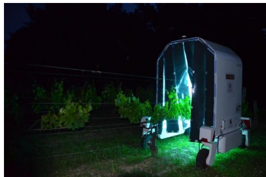
UVC robot in action at Cornell Pathology Vineyards, D. Gadoury, Cornell University
