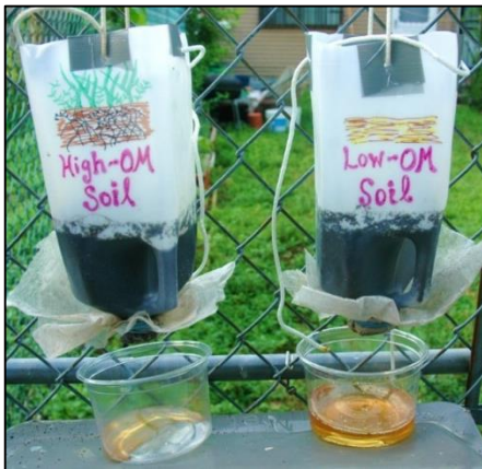
Figure 2. Demonstration illustrating the effect of soil organic matter (SOM) on water-holding capacity:
