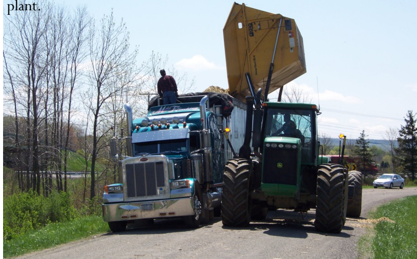
Figure 23: Dumping the willow chips from the large forage dump wagon into the open top chip trailer to be hauled to the power plant.
