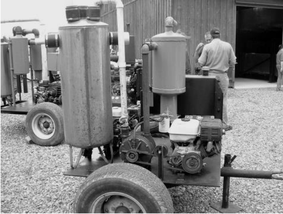
Gas powered vacuum pump on a trailer
