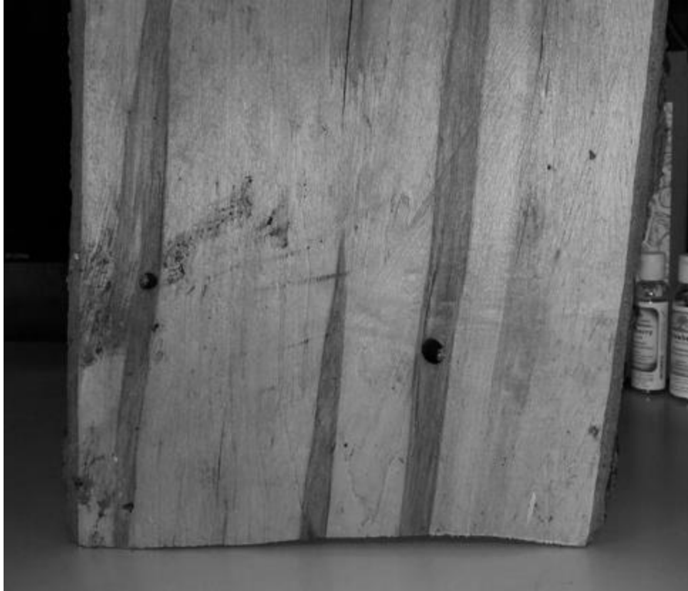
Partitioned wood. Notice how the stain is widest at the taphole narrowest at the ends.
