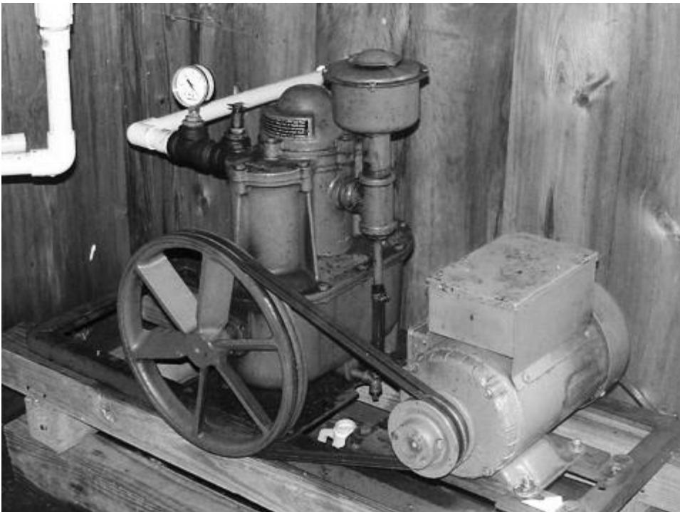
Old dairy vacuum pumps are available very cheap or even free
