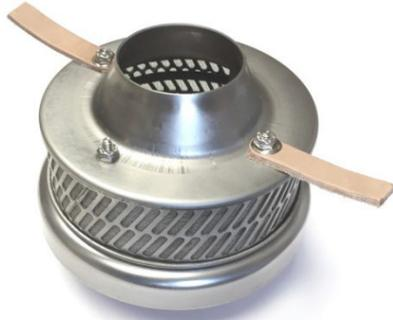
flow control leather straps that cannot be easily seen while spinning; these straps can deliver a painful slap if the operator's hands to get too close to the spinner.
