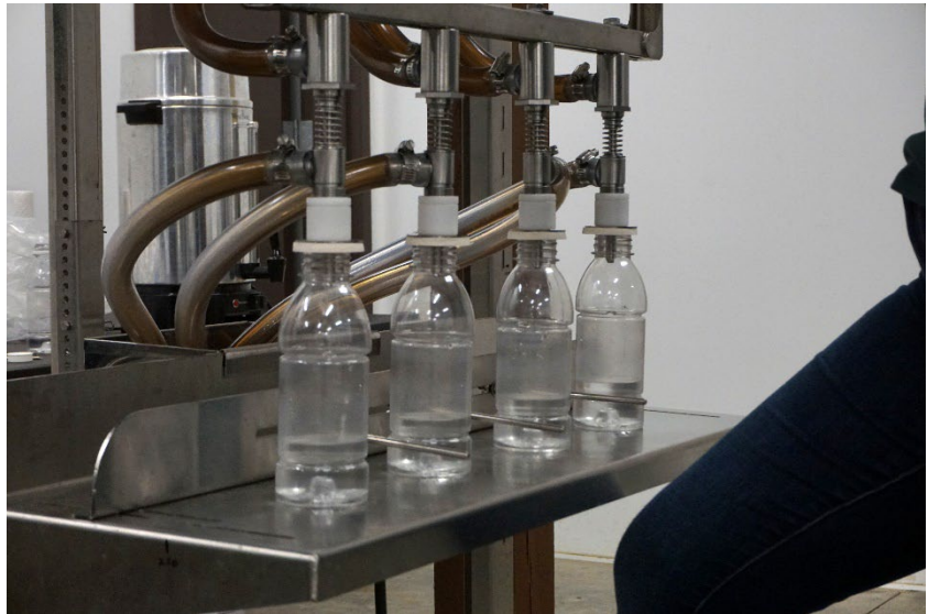
Figure 3. Acidified and thermally treated maple sap bottled using a water jacketed tank. This same unit is used for bottling maple syrup and similar bottling units are common in maple syrup production facilities. Photo by Ailis Clyne.
