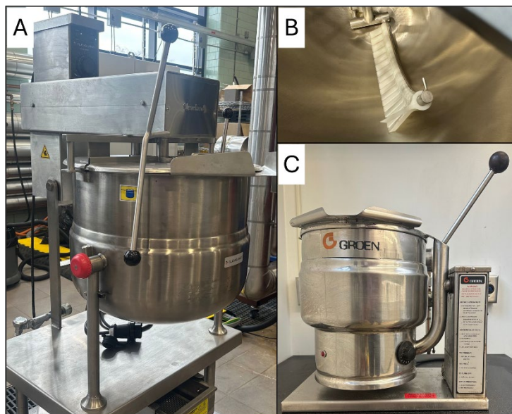
Figure 2. Open Kettle examples, Lee Scraped Surface Open Kettle (A, B) and Groen Steam-Jacketed Kettle (Courtesy of the Seneca Foods Foundation Pilot Plant).
