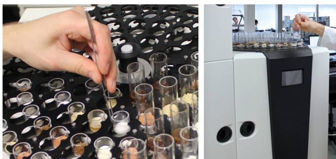
FIGURE 2. Primacs SNC-100 Carbon and Nitrogen Analyzer measures Tot C and N in soil and plant samples.
