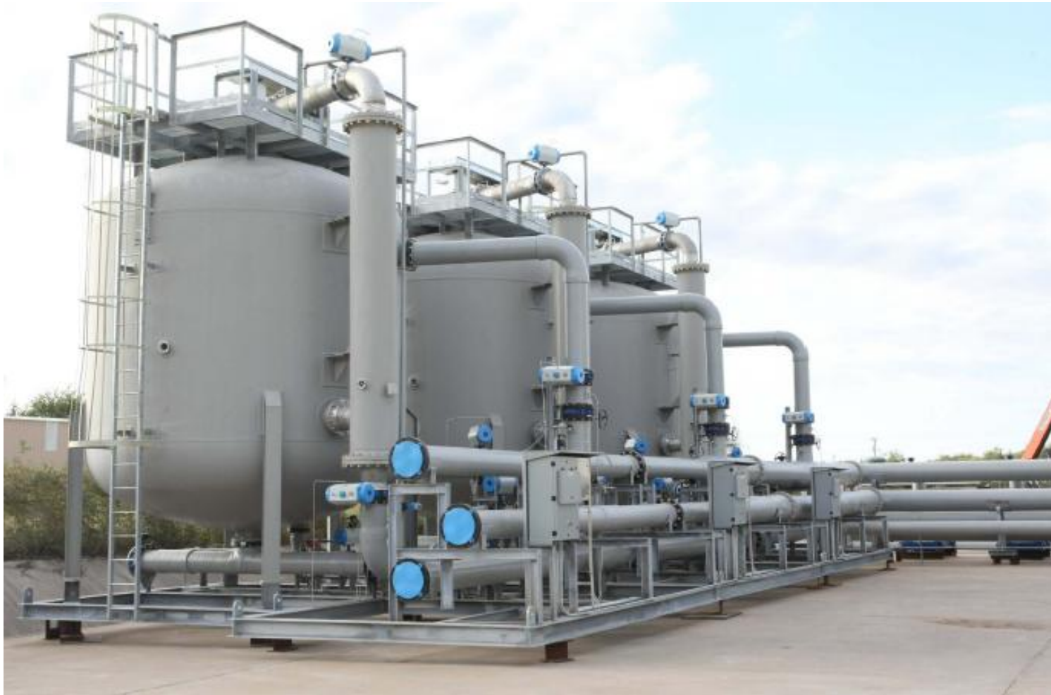
Modern Walnut Shell Filtration Package (Courtesy of Produced Water Society)
