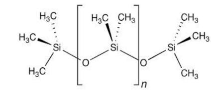
PDMS is widely used to transfer organic& inorganic samples in many labs. For such duty, an ideal PDMS should possess a soft surface to prevent damaging investigated material, appropriate adhesion and leaves minimum residue behind.
