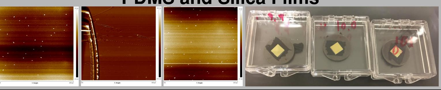
3 sample AFM scans for clean and exposed side. PDMS on gold evaporated silica.
