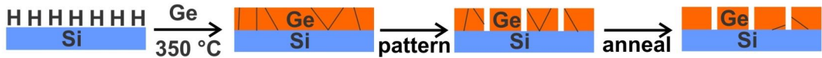
Figure 4.1. Diagram indicating how the patterned virtual Ge substrates were fabricated. The Ge is deposited on H-terminated silicon at 350 \text{ }^\circ\text{C} , patterned using photolithography, and annealed to reduce the dislocation density.
