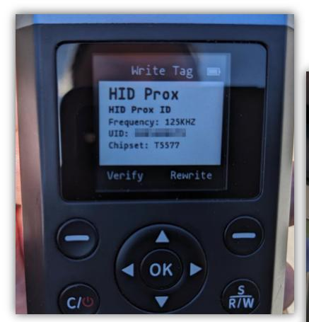
iCopy-XS revealing HID Prox unencrypted RFID
