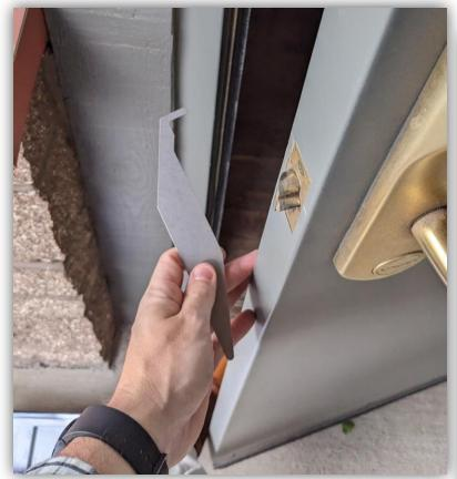
Shim tool made to disengage door latches
