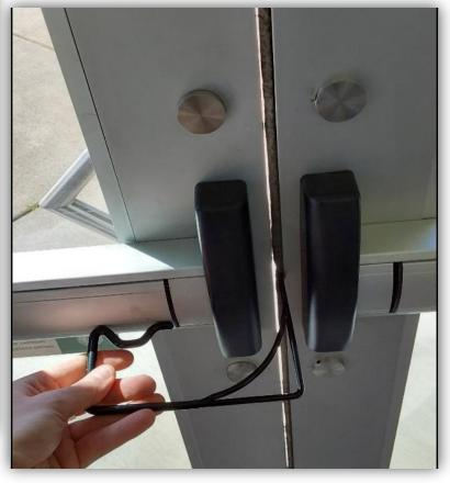
Hook tool made from thick gauge piano wire
