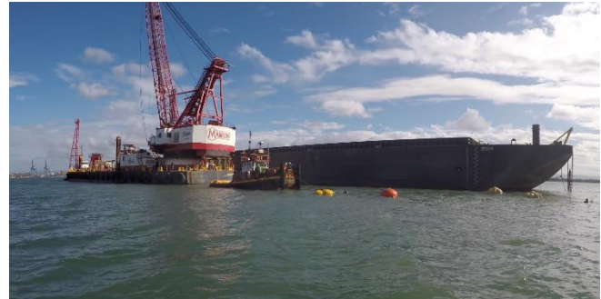
Figure 5. Relocating the shipwreck in mid-water, suspended from eleven lift bags with combined capacity of 22 tons, with tugboat operating in reverse.
