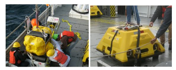
**Fig 2:** Left SIO Abalone Ocean Bottom Seismometer. Right LDEO seismometer, pressure sensor, hydrophone instrument package.
