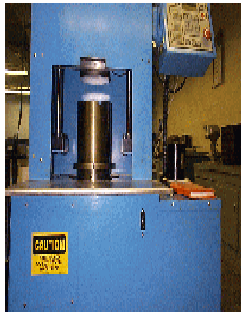
Mold in Compactor Ready to Test
