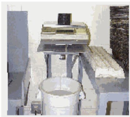
Weighing Specimen in Air
