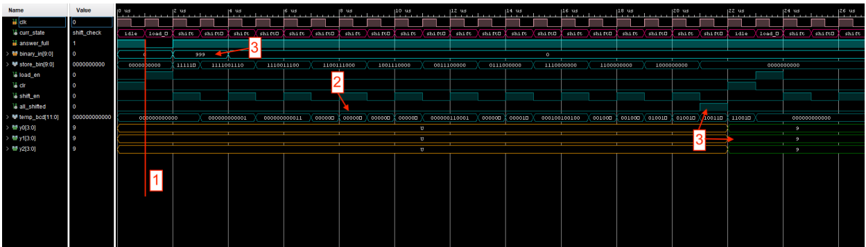
Figure 21: Simulation waveform of the BCD to binary converter. 1)When answer_full goes high converter begins shifting in binary_signal. 2)Between each shift the current BCD variables are checked to see if they are greater than 5. If so, the converter adds 3 to them an continues with the shifts. 3)Upon all shifts being conducted each BCD bin is filled with their respective quantity. In this waveform, the number coming in was 999 and the output was a 9, 9, and 9.
