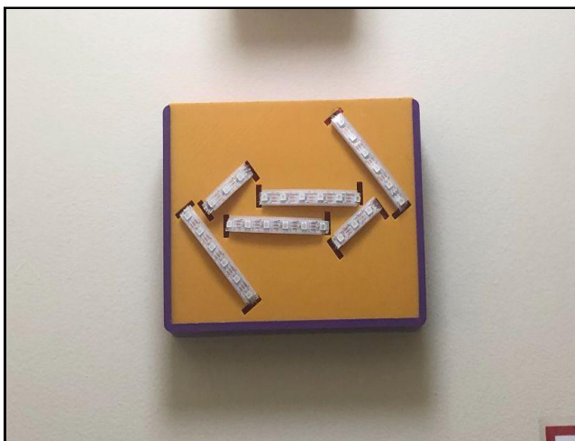
Figure 3: Left: First working prototype with LED strips. Right: Final prototype with wireless connectivity. Note AED subsequently made white to further increase contrast.
