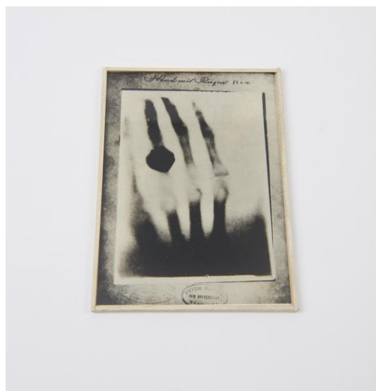
FIG. 1. Original x-ray image of Röntgen's wife's hand [3]. This type of image is created by placing an object in the path of an x-ray spectrum illuminating a barium platinocyanide plate. The plate behind the object becomes fluorescent when exposed to x-rays, but the object's density will hinder the ability of low-frequency x-rays to penetrate it. The obstructed path areas appear darker because only a smaller proportion of x-rays were able to pass through and illuminate the plate in that location. The image left behind is a shadow of sorts, whose darkness is characterized by the density of the object casting it. Close observers may notice that modern x-ray-created images show dense matter as white, and transparent regions as black, which is the opposite of Röntgen's image. Modern x-ray imaging uses a film impregnated with silver halide crystal, which reacts chemically with the film if exposed to x-rays [1]. This chemical reaction turns the film black. Though the image may appear a different color, modern x-ray imaging still depends on the specific energy and size of x-rays predicted by the Duane-Hunt Law as discussed later.
