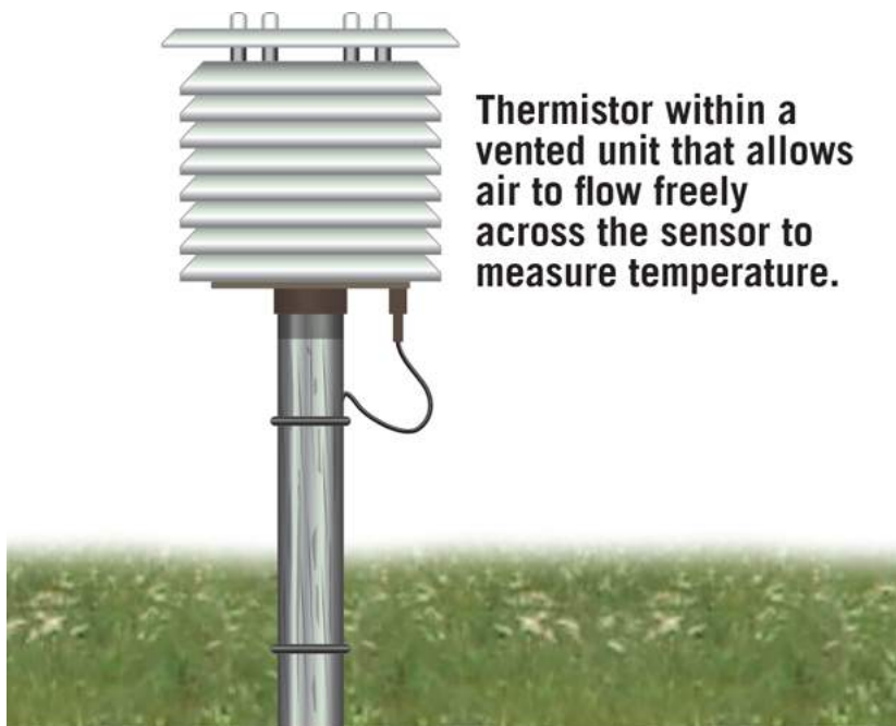
Figure 3.24 Measuring temperature using a thermistor
