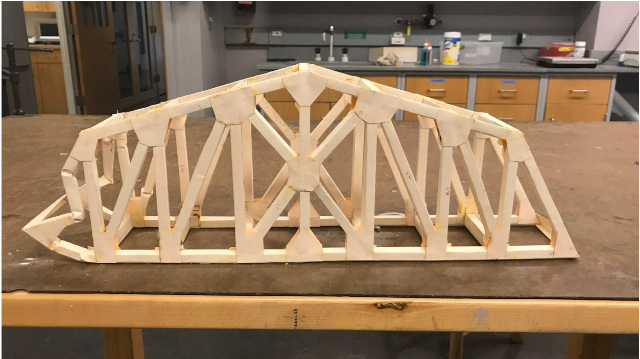
Figure N, Bridge post-testing, with apparent buckling in outermost diagonal member
