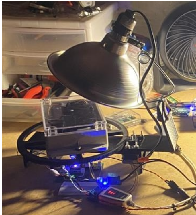
Fig. 16: FOG calibration rig with temperature-controlled enclosure and stepper-motor turntable
