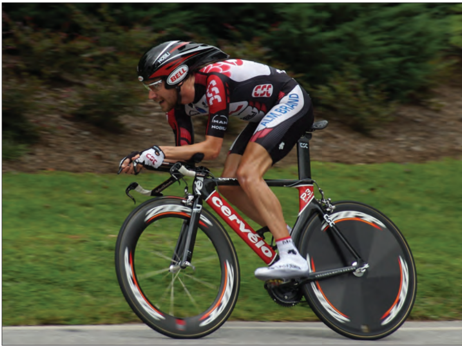
Figure 1: Professional cyclist Dave Zabriskie rides a racing bicycle during a time trial. The solid rear wheel reduces the number of air current eddies which slow cyclists at high speeds.
