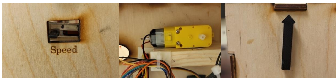
Figure 14: The slider potentiometer attached to the side of the box (left) adjusts the speed of the DC motor (center) which rotates the clock hands (right).
