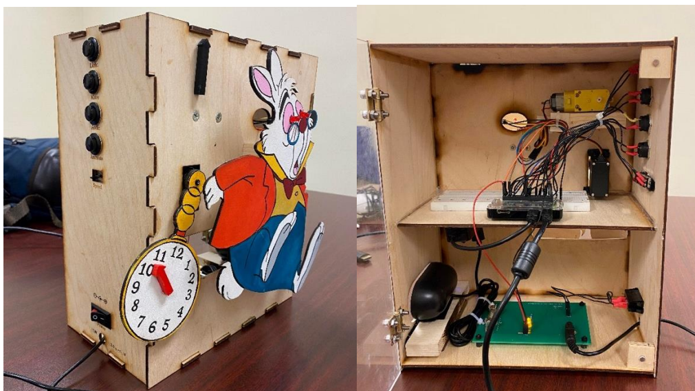
Figure 28: Side view and interior view of our final box. Notable changes: there are wooden squares glued in that hold magnets that secure the door closed, and the DC motor is not using the space originally designed for it (long rectangular hole under shelf), and instead on a shelf in the upper right-hand corner.
