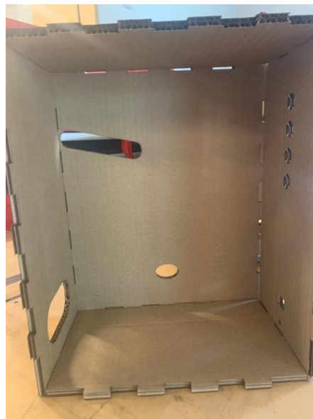
Figure 24: Second box prototype on cardboard, after creating holes and allowances for components. (Of note: the back panel is upside down in this photo.)
