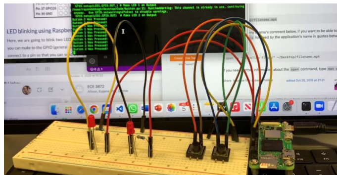
Figure 21: Set up of the Pi based pushbutton simulation.
