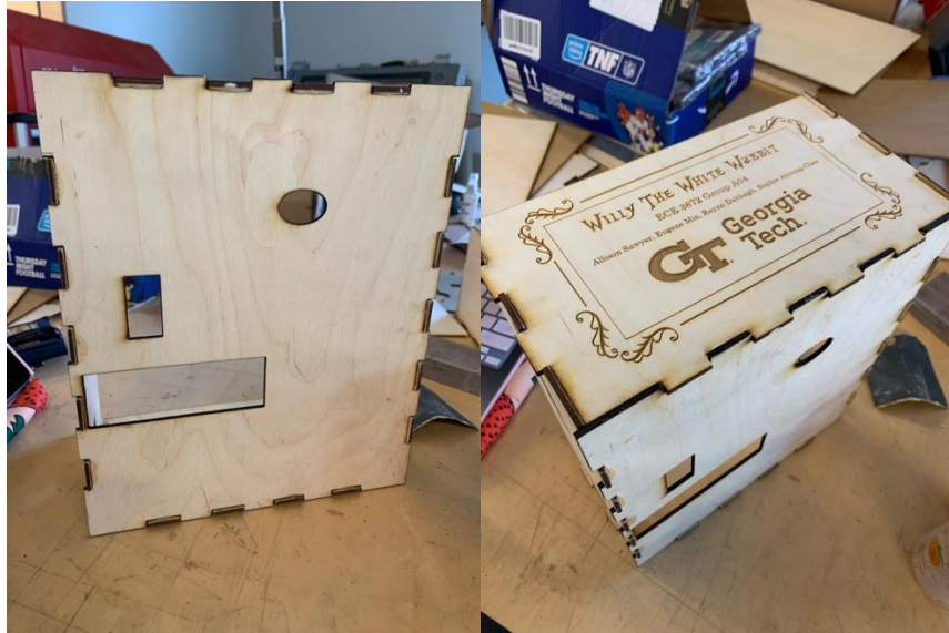
Figure 25: First box prototype on wood, many of these panels are used in the final project. Notable: DC motor to move behind the clock has been enlarged significantly.
