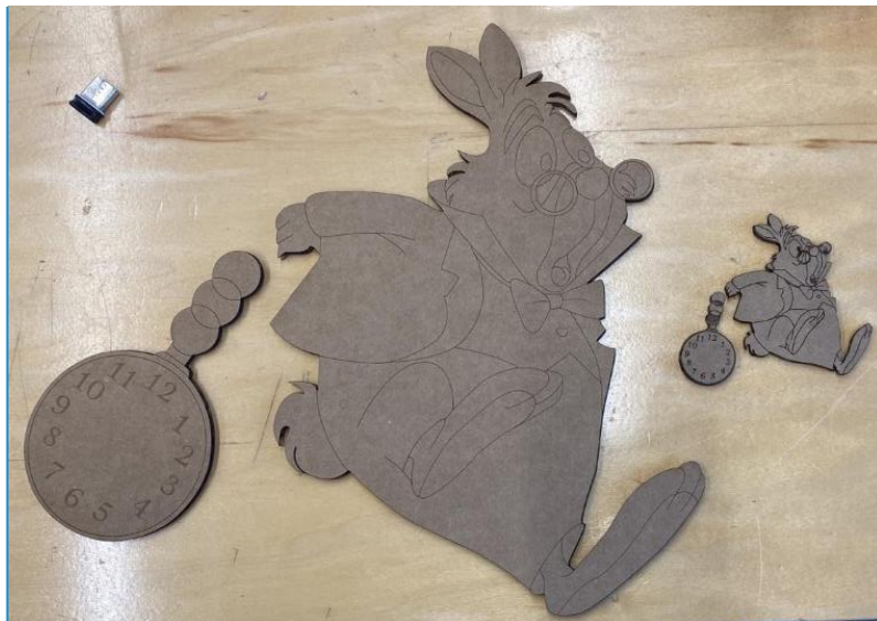
Figure 3: Preliminary laser cut of our design done in cardboard. A 0.25 scaled version was completed first.
