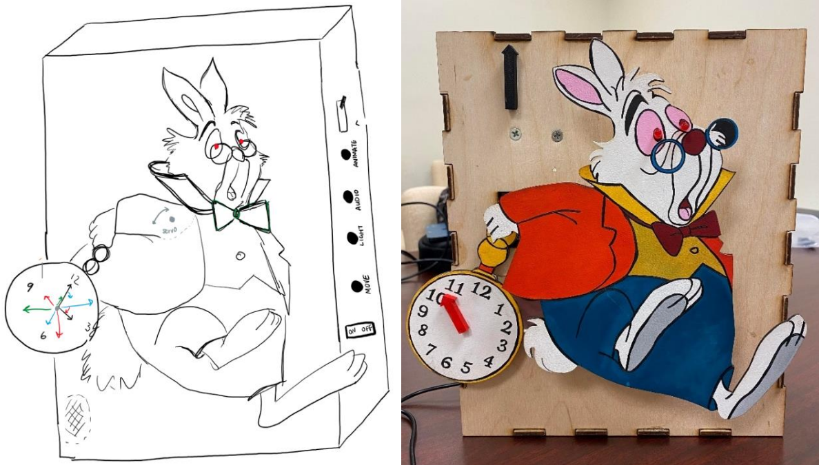
Figure 1: Our second sketch (left) and final design (right) of the White Rabbit. Different from our preliminary design, the rabbit now rests on a vertical box rather than a horizontal box so that our components are not exposed.
