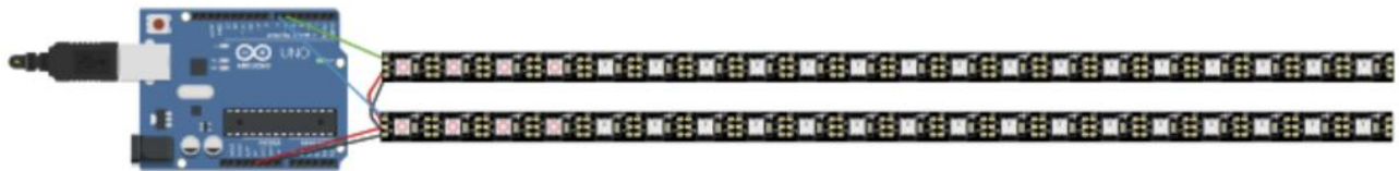
Figure 14. TinkerCad simulation of an Arduino Uno driving two WS2812 LED strips with no additional hardware.
