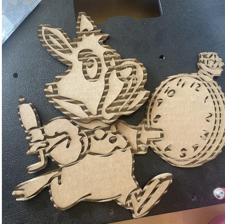
Figure 21. Cardboard laser cut test of rabbit design.
