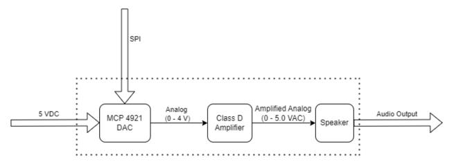
The output of the DAC is not loud enough. As a result, the analog signal gets fed into a Class D Amplifier. The amplified analog signal then gets fed into a speaker which outputs the music/ audio. It was not known when designing whether or not a low-pass filter would be needed. After testing the circuit on a breadboard, the low-pass filter was reducing the noise level significantly. The class D amplifier already contained a low pass filter, so adding an external one was not necessary.
