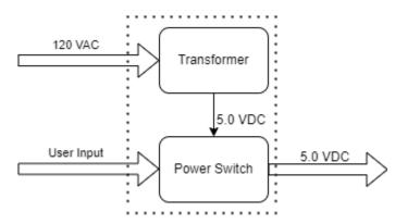
The conversion from 120 VAC to 5 VDC is performed by a 25 W rated transformer with safety circuitry. The entire device contains a user-accessible power switch. When the switch is closed, the 5 VDC can be propagate to the motor driver and Rasberry Pi.
