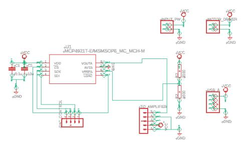
The labels beside the header pins reveal the function of the pins. For example, the pins labeled TO\_AMPLIFIER are used to route the 5VDC to the class D amplifier. The pins labeled USB\_A were connected to a female USB type A breakout board. A USB to mini-USB cable provided power to the Raspberry Pi. This approach of supplying power to the Pi was selected over using the Vin pins because safety circuitry is embedded in power provided through the female mini-USB port on the Raspberry Pi 0 w.
