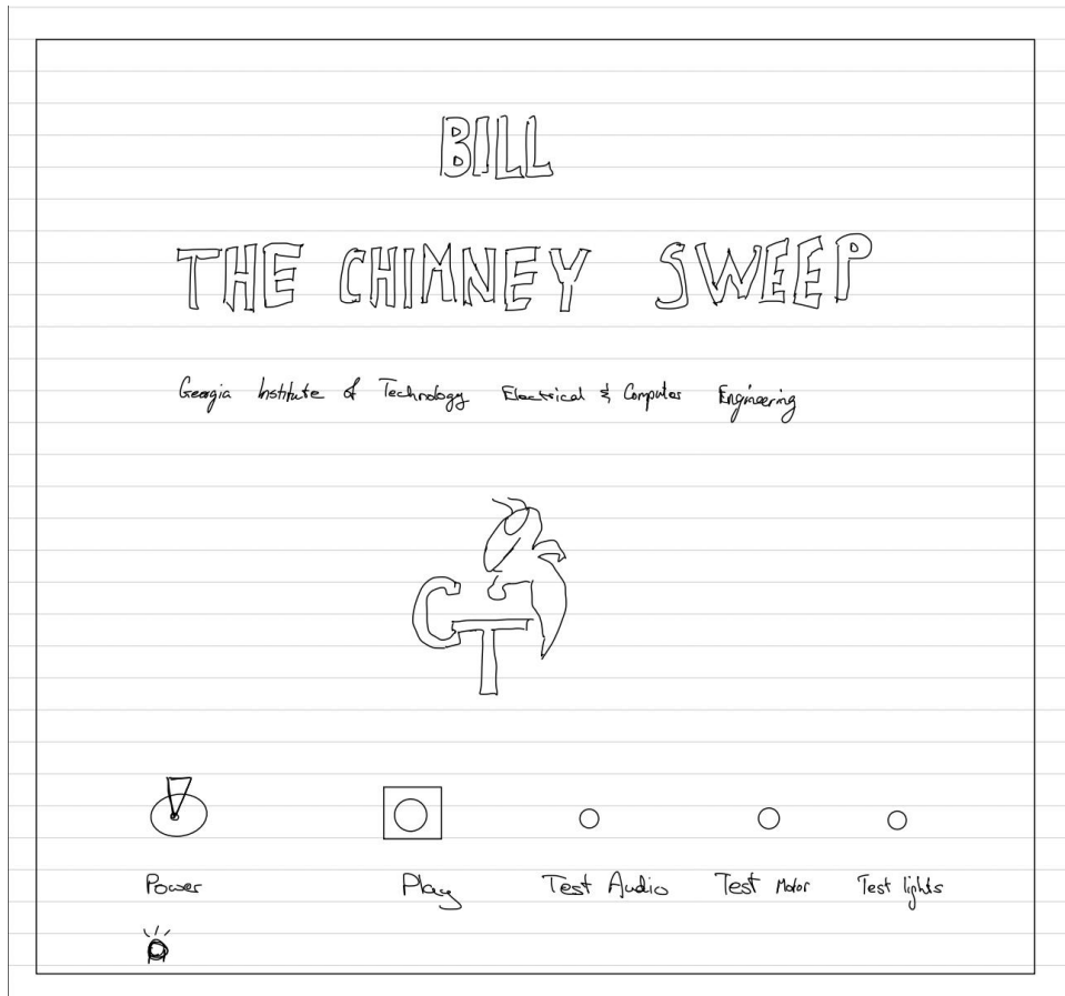
Figure 15: Rough sketch of the front face of the box showing button layout
