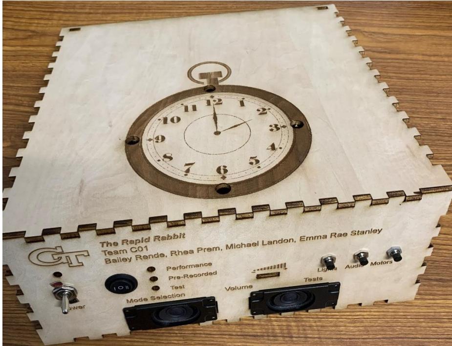
Figure 21: Laser Cut Wood Prototype of Robot Base
