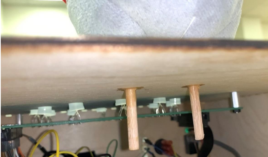
Figure 23: Wooden Dowels to Secure Rabbit to Box
