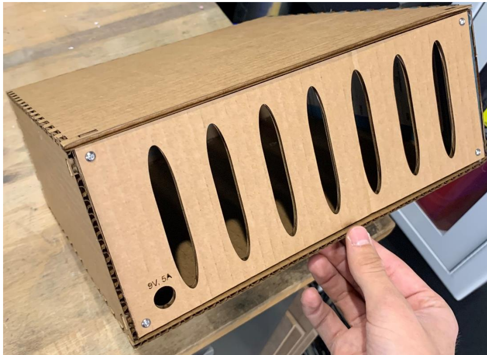
Figure 20: Laser Cut Cardboard Prototype of Robot Base
