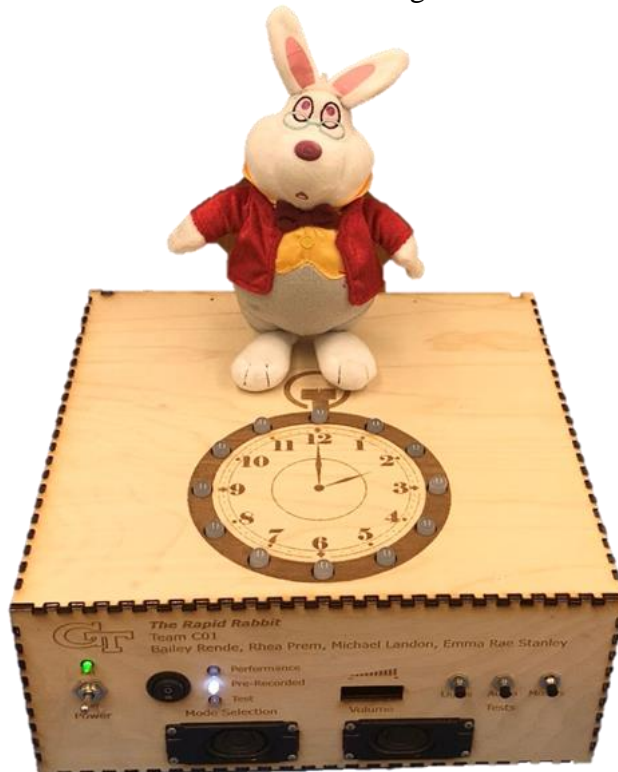
Figure 22: Laser Cut Wood of Robot Base Final Design
