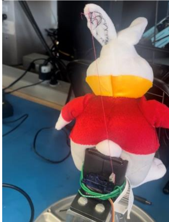
Figure 27: Thread Attached to Ear to Move Up and Down via Servo
