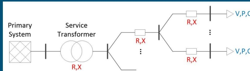
Linear regression to find  $R_1$ ,  $R_2$ ,  $X_1$ ,  $X_2$  values which best fit the  $V_1$ - $V_2$  fluctuations
