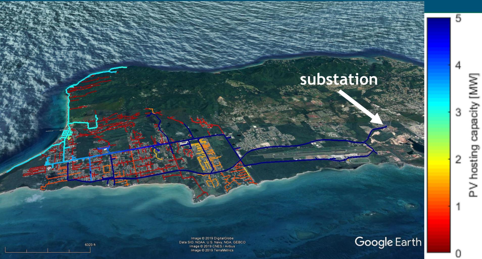
Modeling many PV interconnections on a feeder is difficult: usually only 1 (or no) solar irradiance measurement available near a feeder.
