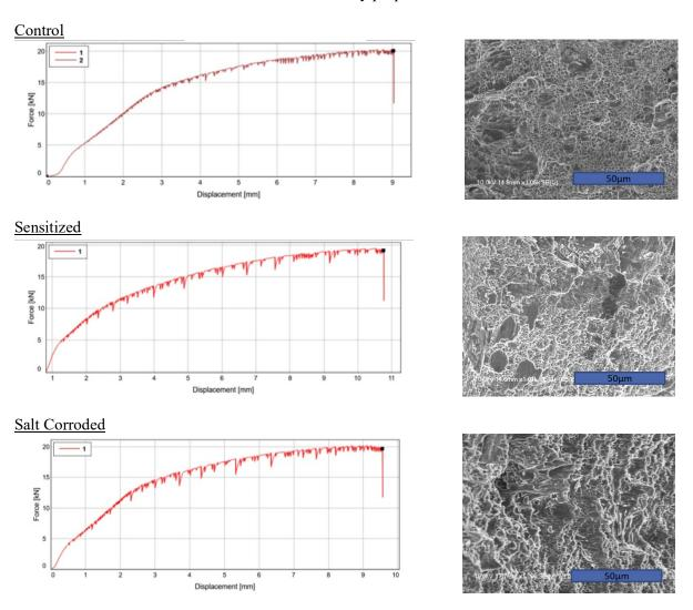
Salt Corroded and Sensitized
