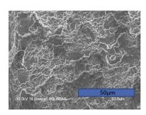
When observing the graphs, there is an increase in the amount of spikes on the graphs based off the order given above. These spikes account for dislocation diffusion. During the tensile test, the dislocations get stuck on the magnesium molecules, so it requires more force until it breaks free. The SEM Images also tend to show that the metal increasingly becomes more brittle after it is exposed to heat and salt water.
