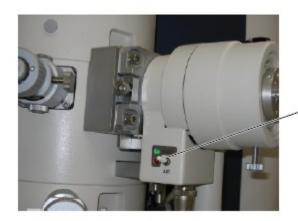
When the specimen holder has returned to the inserting position, turn the EVAC-AIR switch to AIR.
