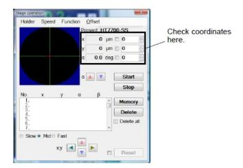
**NOTE:** If the specimen holder is taken out other than in the home position, the objective lens and adjacent parts may be damaged by the specimen holder.
