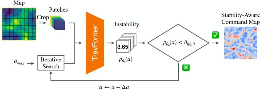
$v_{m_{\text{loc}}}^* = \max \left\{ v \mid \text{VaR}\left(p_{\theta_{\delta}}(m_{\text{loc}}, [v, 0]), \alpha\right) < \delta_{\text{limit}} \right\}$  $\omega_{m_{\text{loc}}}^* = \max \left\{ \omega \mid \text{VaR}\left( p_{\theta_{\delta}}(m_{\text{loc}}, [0, \omega]), \alpha \right) < \delta_{\text{limit}} \right\}$
