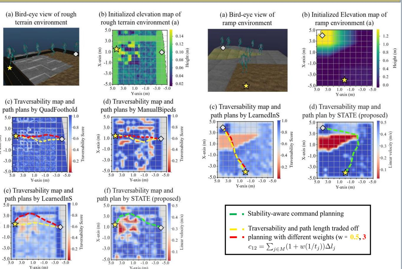
The proposed method properly estimates the risk of dangerous area in rough terrain and robustly produces safe global path plans across varying environments.
