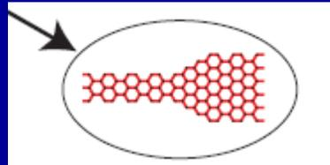
Smoothness leads to enhanced confinement and resonant tunneling – quantum dot
