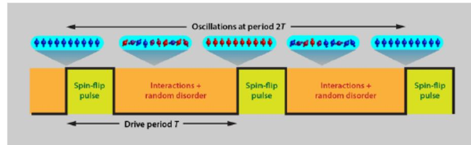
**Figure 1:** Yao *et al.* [7] have developed a blueprint for creating a time crystal and a method for detecting it, which has been followed by two experimental groups [8, 9]. Quantum spins are subjected to imperfect spin-flip driving pulses and then allowed to interact with each other in the presence of strong random disorder in the local
