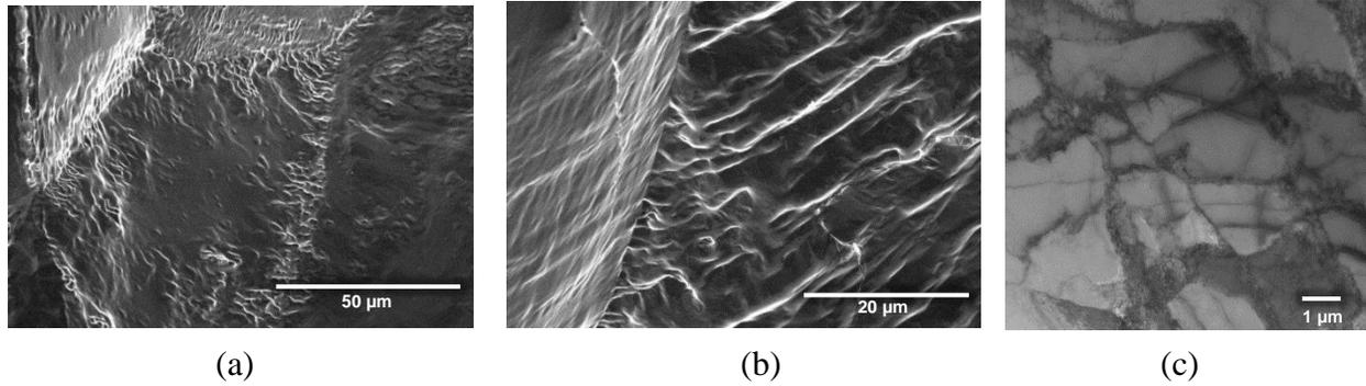
Figure 7. After 1000 cycles, (a) SEM image of GB morphology showing extensive irregularly shaped lumps on GBs, (b) SEM image of triple point extrusions, and (c) bright field TEM image of well-defined dislocation cells formed.
