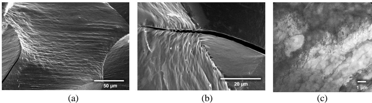
Figure 6. After 100 cycles, (a) SEM image of GB structure showing extensive deformation ledge and lump formation, (b) SEM image showing extrusions forming preferentially at triple junctions, and (c) Bright-field TEM image of early stages of dislocation cell formation.
