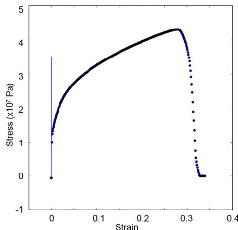
Figure 2. Stress-strain curve obtained from tensile test of the same specimens used for fatigue tests. The yield point is around 12 MPa.
