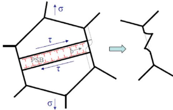
Figure 1. PSB-GB interaction: irreversible slip and dislocation pile-up at GB causes GB roughening by extrusion formation. Image modified and used with permission from [5].
