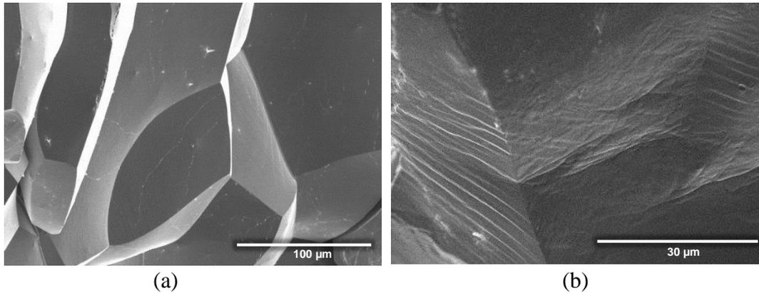
Figure 3. SEM images of the as-annealed GB morphology after liquid Ga embrittlement showing (a) smooth, featureless GBs representative of the majority of the observations and (b) limited areas of ledges formed on the GB faces.
