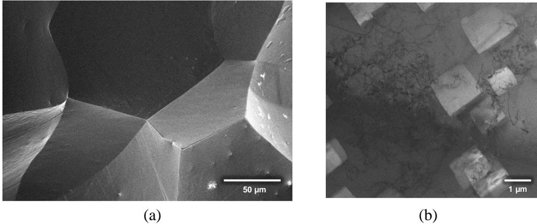
Figure 5. After 1 cycle, (a) SEM image of GB morphology, similar to as-annealed condition and (b) bright field TEM image of randomly entangled dislocations
