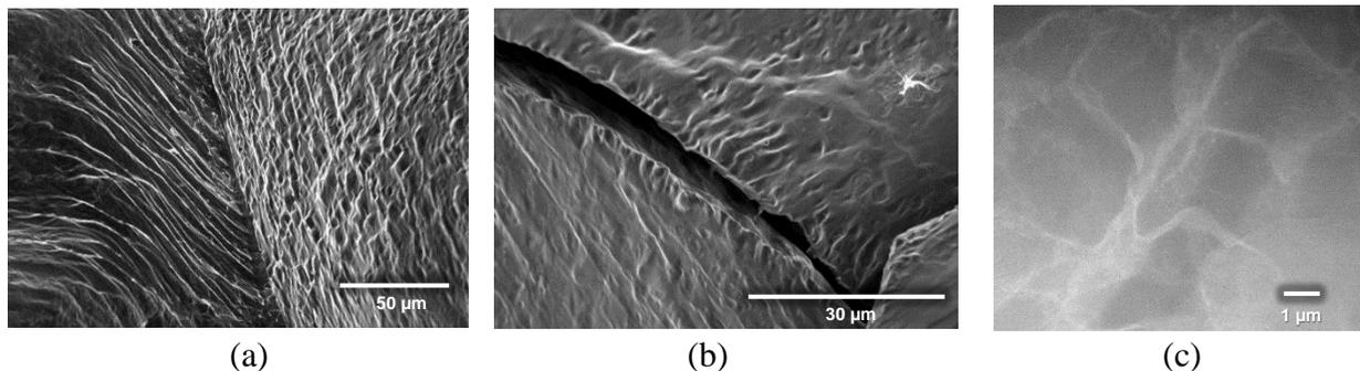
Figure 4. SEM images of (a) GB covered by ledges and (b) extrusions at triple junctions after failure. (c) Well defined dislocation cells after failure under low cycle fatigue, imaged by STEM.
