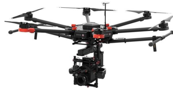
DJI Matrice M600 Industrial Drone: Currently used for human piloted radiation mapping at INL
