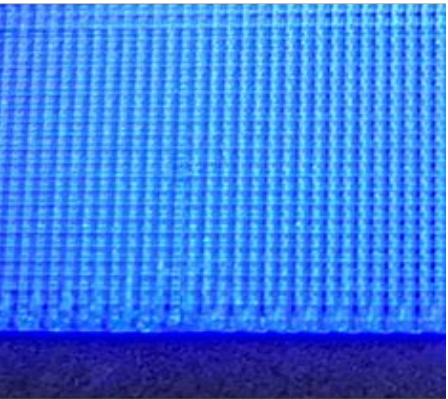
Fine structures: currently printing 250 microns, going down to 50 only requires more filtering
