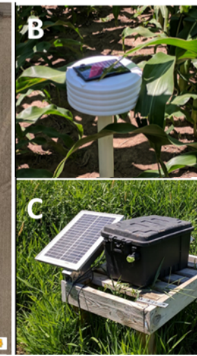
Solar powered Raspberry PI gateway
