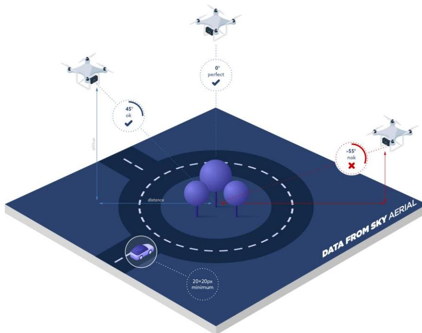
**Figure 1. The incidence angle of the drone should be below 55 degrees**
