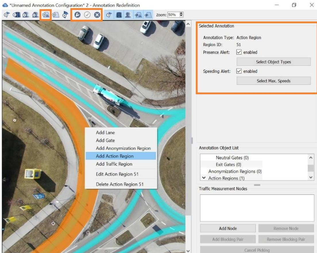
**Figure 12. Set up an Action Region (Orange Area) in One Intersection Approach**
