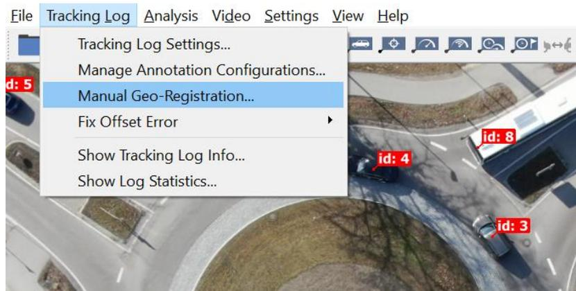
**Figure 4. Conduct Geo-registration in DFS Viewer**
