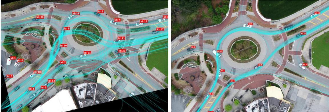
**Figure 2. Vehicle Trajectory Data Extracted from Drone Videos Captured under High Wind Condition (left) vs. Low Wind Condition (right)**
