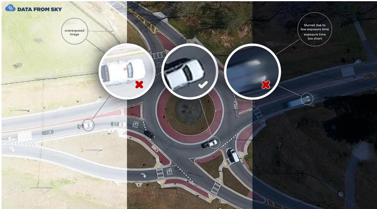
**Figure 3. Three situations – not ok: too bright (left), ok: ideal (center), not ok: blurred due to low exposure time (right)**
