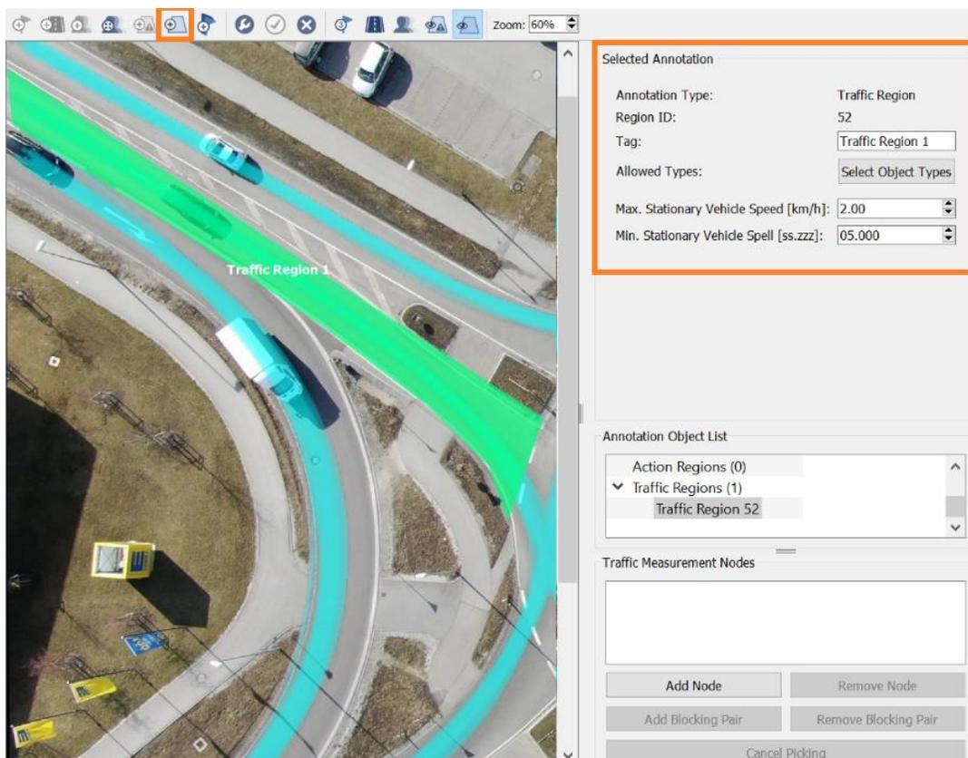
**Figure 13. Set up a Traffic Region (Green Area) in One Intersection Approach**
