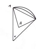
Now if we have an arc of a circle of radius s, cutting out an angle  $0 < \beta < \pi$  from its center, subsuming a chord AB as in this figure below, the length of a chord AB is  $2s \sin(\beta/2)$ .
