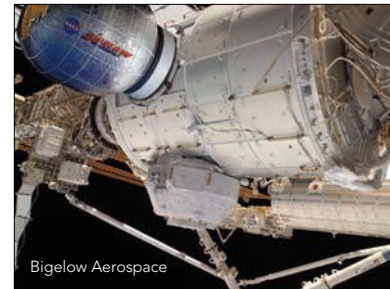
Artist's rendering of the Bigelow Expandable Activity Module attached to the International Space Station. The module will be launched to the space station on a SpaceX flight.
