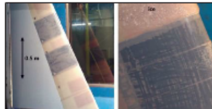
Anticing was demonstrated on unmanned air system aerosurface. Left: Aerosurface (white) with GFR-modified regions. Right: Delicing during ice tunnel testing. Courtesy: MIT and NDC.
