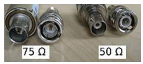
be coloured red in 75 ohm connectors, and while this is occasionally implemented, it did not become standard. The 75 ohm connectors are typically specified for use at frequencies up to 2 GHz. 75 ohm BNC connectors are primarily used in Video (particularly HD video signals) and DS3 Telco central office applications. Many VHF receivers use 75 ohm antenna inputs, so they often used 75 ohm BNC connectors.
