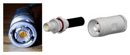
Early triaxial connectors were designed with just an extra inner conductor, but later triaxial connectors also include a three-lug arrangement to rule out an accidental forced mating with a BNC connector. Adaptors exist to allow some interconnection possibilities between triaxial and BNC connectors.
