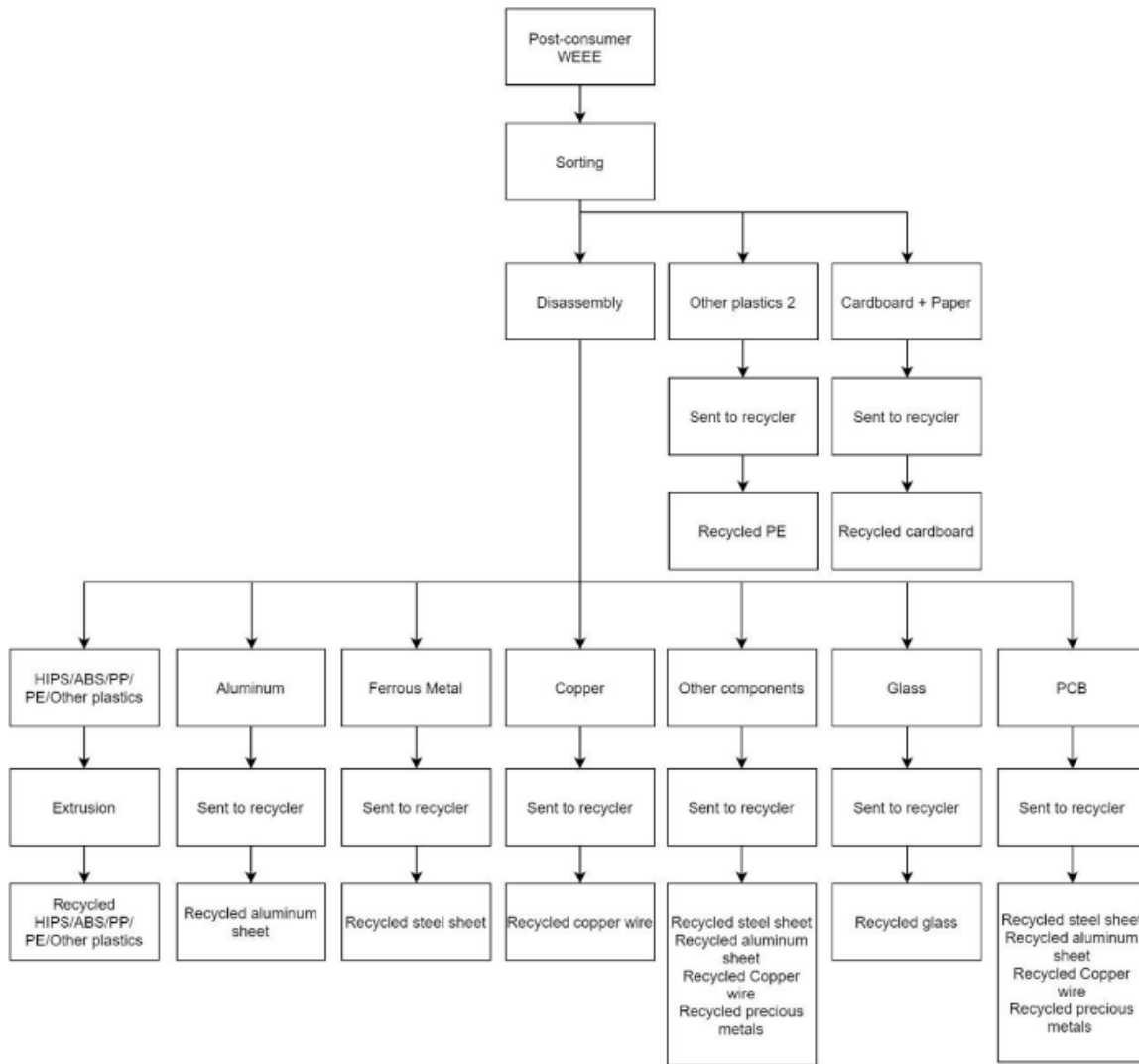
Figure 1: Flex in Sorocaba Process Flow. Source: CSA Registries
