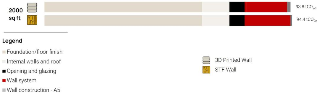
Figure 7: Embodied carbon of the two modeled structures. Results from Tally.
