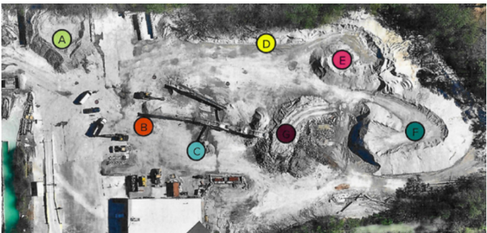
Figure 2. Plant site with stockpiles that were used for this study. The carbon uptake of concrete is highest at the end-of-life phase, when it is crushed and the surface area is maximized. A model is developed to measure the carbon uptake of concrete at end-of-life, accounting for time, space, and particle size.
