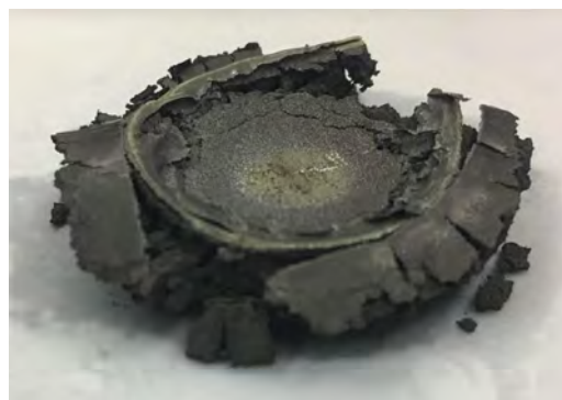
Figure 3. Cylindrical sample after axial compression test.
